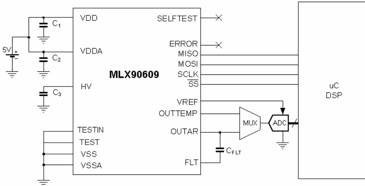
**Figure 6-1. MLX90609 with simultaneous analog and digital output**
