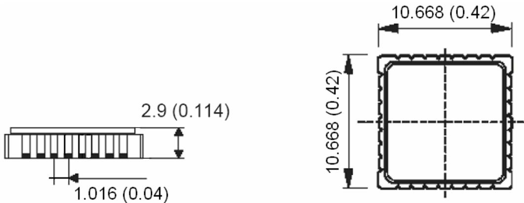
**Figure 9-2. Side and Top View of the MLX90609**
