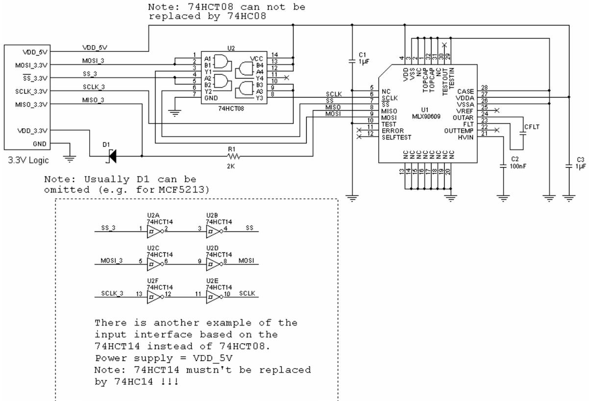
**Figure 6-4. Possible interfacing with 3.3V  $\mu$ C**
