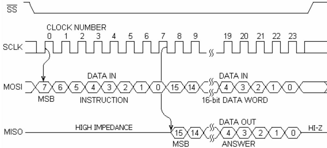
**Figure 5-2. Serial Exchange Sequence (full answer reading)**
