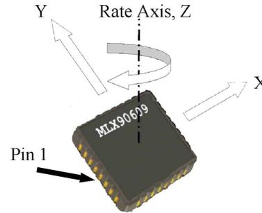
The MLX90609 has various build in features to support automotive and high volume applications (built-in on demand and non disruptive continuous self test, serial number in EEPROM...). These types of applications need close cooperation between the customer and Melexis. Please contact Melexis in case you have such an application.
